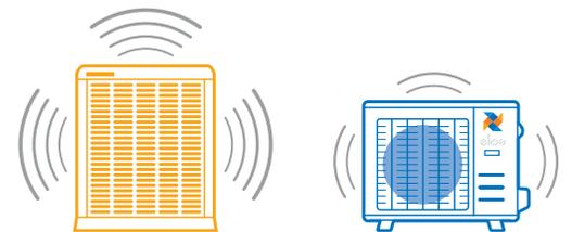
Traditional central system: 73 dB(A) Central-Elios system: 58 dB(A)
